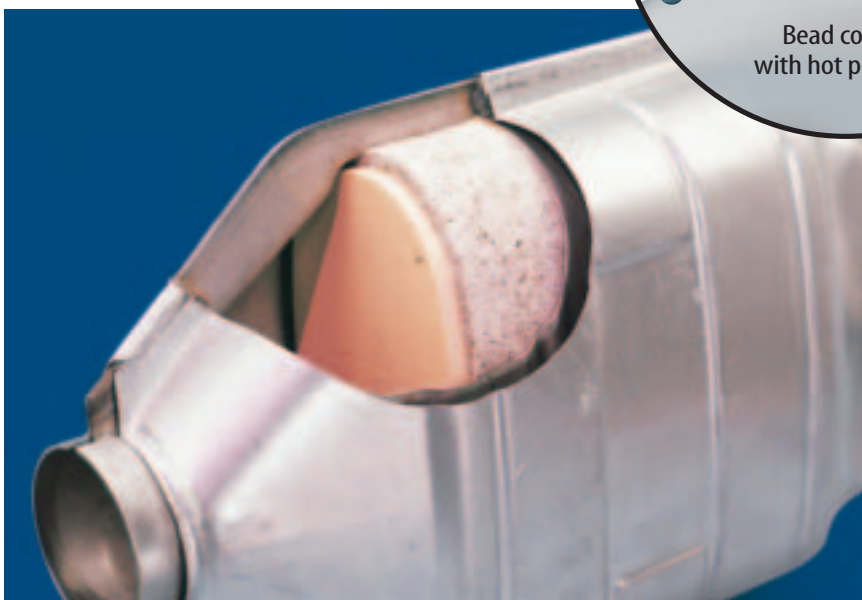
Figure 19 Catalytic converters help to complete combustion of fuel. Hot exhaust gases pass over the surfaces of metal-coated beads. On the surface of the beads, carbon monoxide and hydrocarbons are converted to \text{CO}_2 and \text{H}_2\text{O} .
