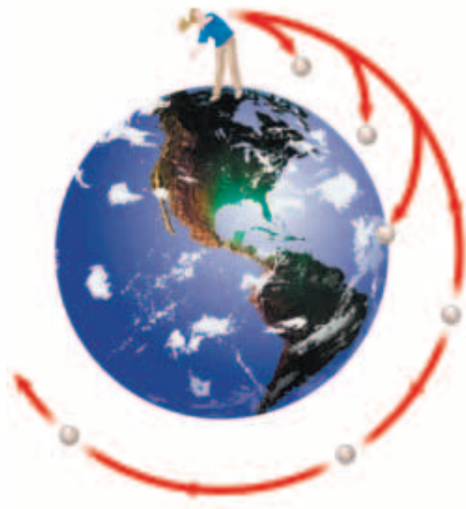
Figure 11 The faster a ball is thrown, the farther it travels before gravity pulls it to Earth. If the ball is traveling fast enough, Earth's surface curves away from it as fast as it falls downward. Then the ball never hits the ground.
