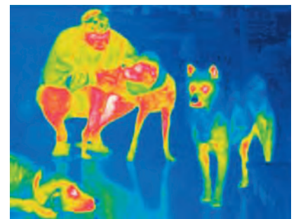
▲ Warm objects emit infrared light, which is invisible to the eye but can be captured on film or by detectors to produce an infrared photograph. (© Sierra Pacific Innovations. All rights reserved. SPI CORP, www.x20.org.)
