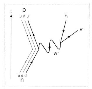
The Feynman diagram for beta decay of a neutron into a proton, electron, and electron antineutrino via an intermediate heavy W boson
