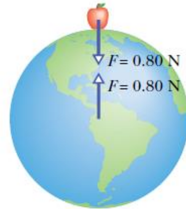
Fig. 13-3 The apple pulls up on Earth just as hard as Earth pulls down on the apple.
