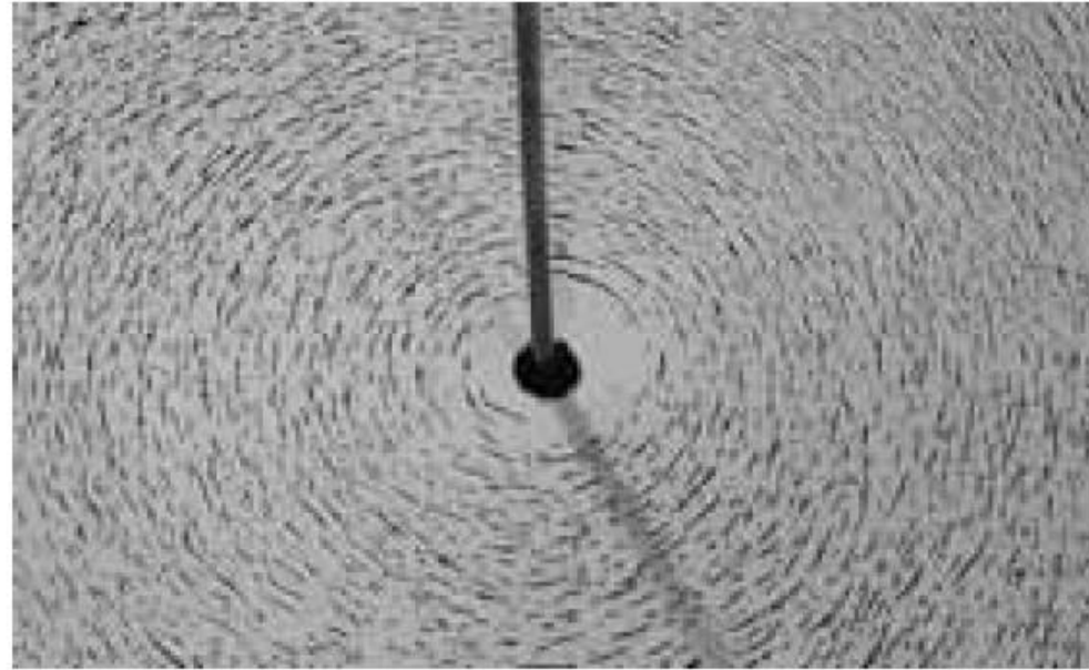
Fig. 29-3 Iron filings that have been sprinkled onto cardboard collect in concentric circles when current is sent through the central wire. The alignment, which is along magnetic field lines, is caused by the magnetic field produced by the current. ( Courtesy Education Development Center )
