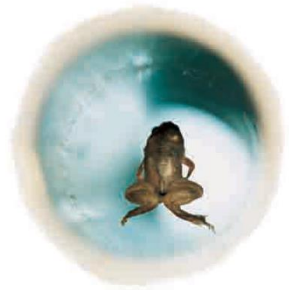
Fig. 32-13 An overhead view of a frog that is being levitated in a magnetic field produced by current in a vertical solenoid below the frog. (Courtesy A. K. Gein, High Field Magnet Laboratory, University of Nijmegen, The Netherlands)
